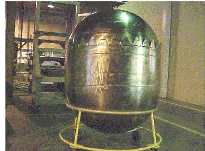
Commercial Cryogenic Tank; rated 250 psi
